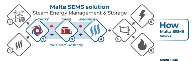
Input, Variable Power and Residual Heat. Electricity is collected from renewables or excess grid power. Residual heat can also be collected when available.
